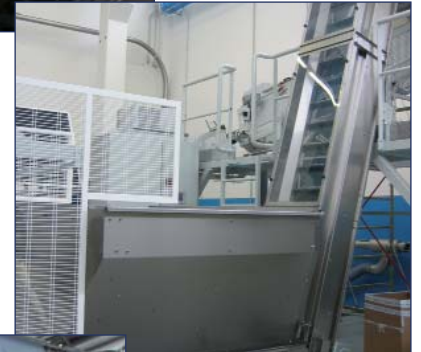
hopper to collect preforms complete with elevator
