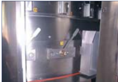
phase number 1 View of the lever fixing system: open position of the separator
