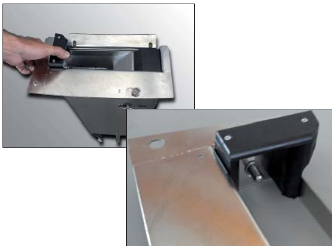
View of the cradle regulation system in preset positions: the holes can easily be seen.
